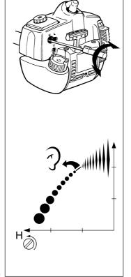
before adjusting the high speed needle. The high speed needle is adjusted correctly when the machine 'splatters' a little . If the machine smokes heavily at the same time as it 'splatters' heavily the adjustment is too rich.
